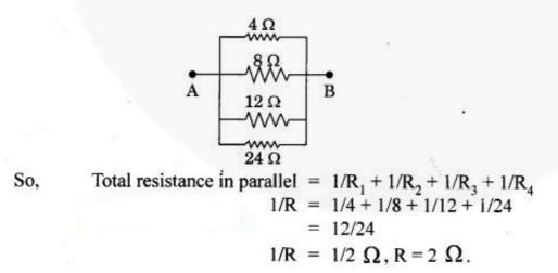
Resistance is lowest when connected in parallel.
