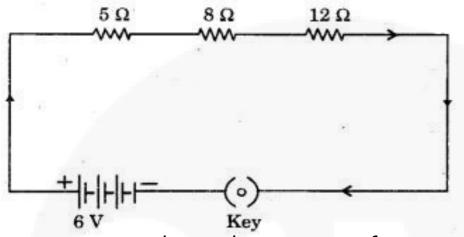
Question 2. Redraw the circuit of question 1, putting in an ammeter to measure the current through the resistors and a voltmeter to measure the potential difference across the 12  $\Omega$  resistor. What would be the readings in the ammeter and the voltmeter?
