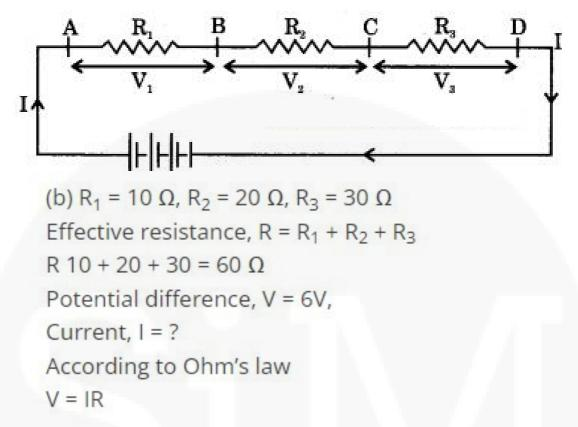
Question 9. Find the resistance between points A and B in the circuit diagram given below
