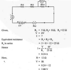
Hence, reading in the ammeter would be 0.24 A and reading in voltmeter would be 2.88 V.
