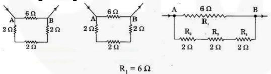
Ans. R<sub>2</sub>, R<sub>3</sub>, R<sub>4</sub> are in series and have resultant resistance R R' = R<sub>2</sub> + R<sub>3</sub> + R<sub>4</sub> = 2 + 2 + 2 = 6  $\Omega$ R' is in parallel combination with R<sub>1</sub>  $\therefore$  Resultant resistance of the circuit (R')  $\Rightarrow \frac{1}{R} = \frac{1}{R_1} + \frac{1}{R_1} = \frac{1}{6} + \frac{1}{6} = \frac{2}{6} = \frac{1}{3}$  $\therefore$  Resultance, R = 3  $\Omega$ .
